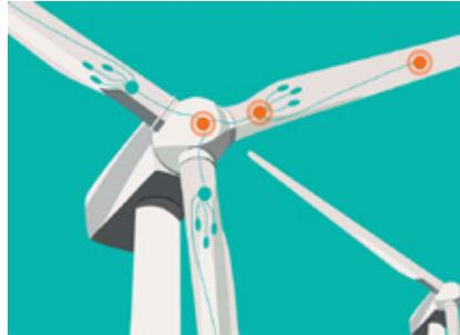
electromagnetic interference and damage caused by lightning strikes, in contrast to electrical systems. Due to the high cycle durability of fibre-optic sensors, a very long service life of the system is achieved. Retrofit installation is possible in less than one day per turbine.
