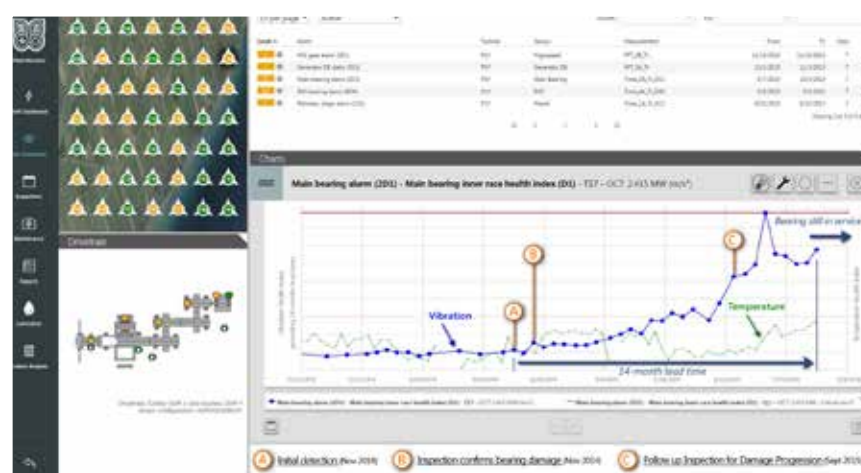
Figure 1. Romax InSight Fleet Monitor™ hardware-independent Cloud-based predictive maintenance software tracking main bearing damage with over a year's lead time on the failure using advanced algorithms applied to the raw vibration data feed. Temperature provides only late stage warning.
