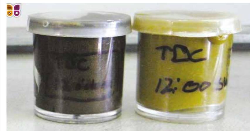
Samples showing grease condition before and after flushing. Fresh grease improve lubrication conditions and extending bearing life
