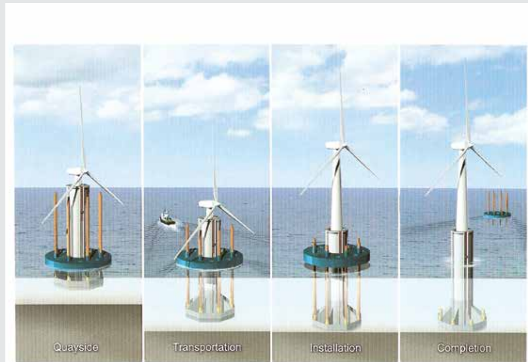
DTI-50 Deepwater Turbine Installation 50 - concrete base
