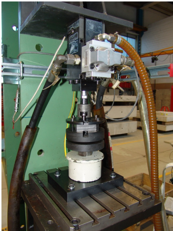
Figure 14. Servo-hydraulic test setup for tension fatigue tests
