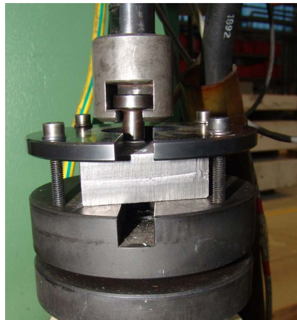
Figure 14. Servo-hydraulic test setup for tension fatigue tests
